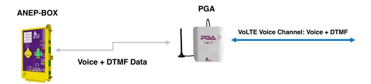
By enabling IP VoLTE mode, the PGA gateway converts DTMF signals for transmission over the data channel.
